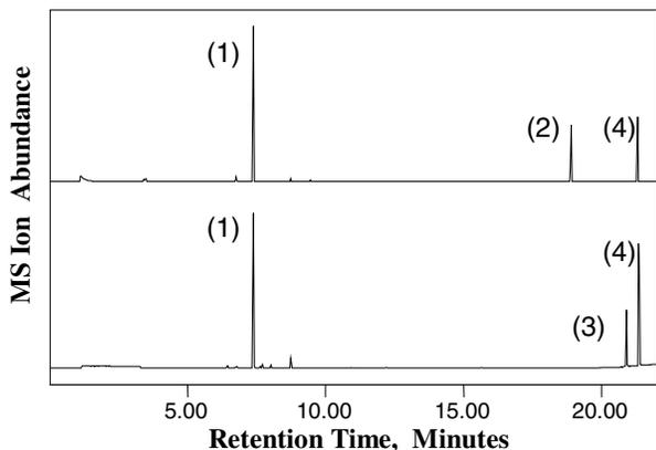
**Figure 3.** TD/GC/MS of pellets (top) and fractured PC part (bottom). (1) chlorobenzene; (2) triphenylphosphine; (3) triphenylphosphineoxide; (4) benzotriazole alkyl phenol.
