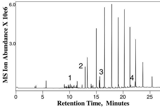
**Figure 7.** TD/GC/MS of unknown PE and candidate sources. (1) hydrocarbons; (2) antioxidant #1; (3) first peak – cyclic compound MW 196; (4) first peak – antioxidant #2.
