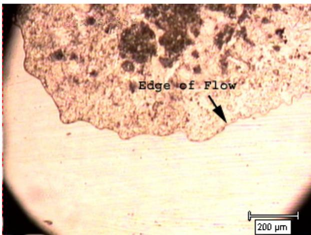
**Figure 9.** Photo of a sealant in IR diamond cell showing the flow front of liquid in the sealant.
