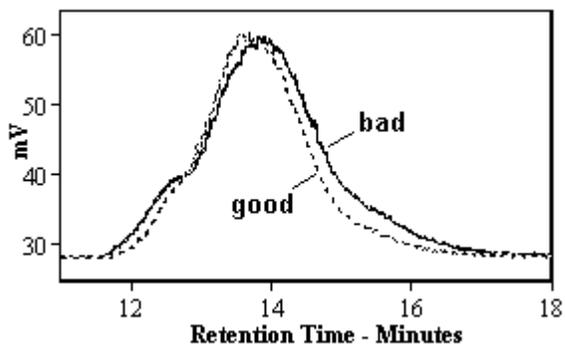
**Figure 1.** GPC of good and bad lots of polymer regarding processing for a coating application.
