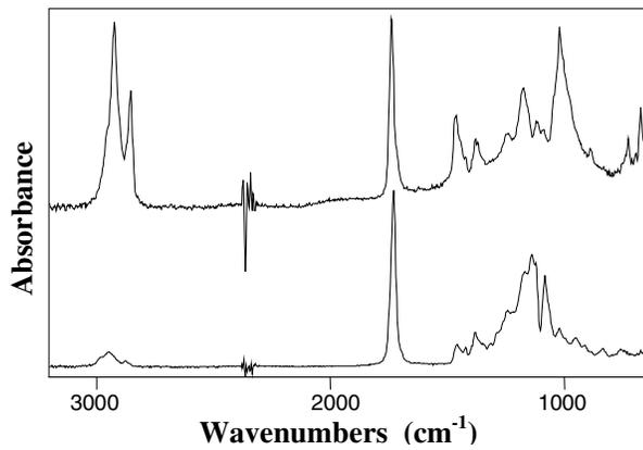
**Figure 8.** IR spectra of non-leaking (top) and leaking sealants (bottom).
