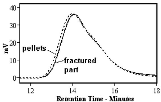
**Figure 2.** GPC of pellets and fractured PC part.
