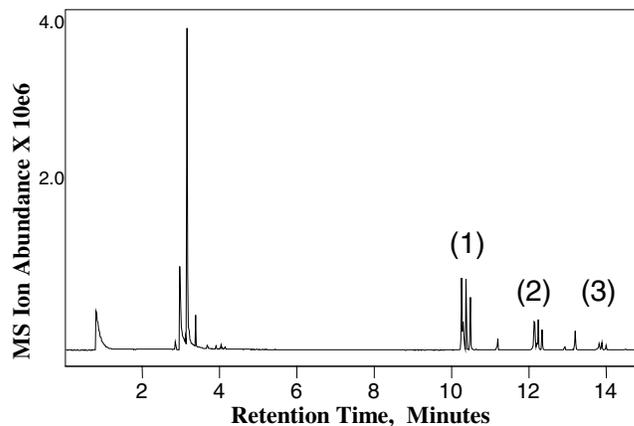
**Figure 6.** TD/GC/MS of particle caught on extruder screen. (1) dodecene isomers; (2) tetradecene isomers; (3) hexadecene isomers.
