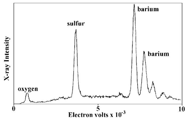
**Figure 5.** SEM-EDX of undispersed particle.
