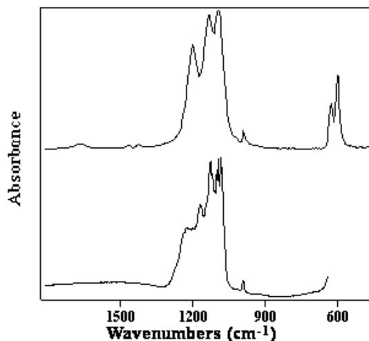
**Figure 4.** IR spectrum of undispersed particle (bottom) and reference spectrum of barium sulfate (top).
